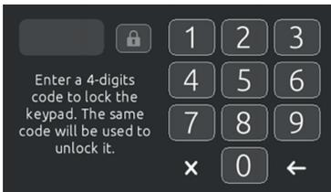
If the user intends to use the lock, he/she is prompted by the system to fill in a 4-digit code. The same code will be required to unlock the keypad.
