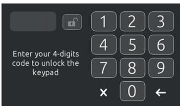
With the next use, the system will again request a 4-digit code (it does not have to be identical). It is possible to unlock the keypad with a universal code (3732), or through an overall reset of the keypad.
