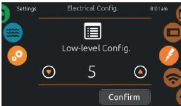
If you want to change the configuration, the number of phases and input current of the Hot tub system, slide the right selection circle until the icon Electrical configuration is highlighted in the centre.
